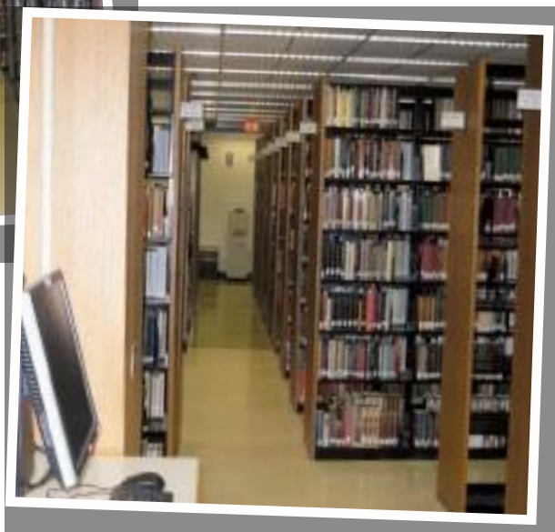
By decreasing the cross aisle from 72" to 42" the library was able to add an additional 13,000 volumes of capacity. The existing shelving was cut from 36" to 30" by the compact shelving installer. This alone saved the library over $12,000 in shelving costs.
